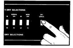
The OFF/CANCEL Button allows you to stop the dryer to check the load, clean the lint screen, or to change the drying selection.
